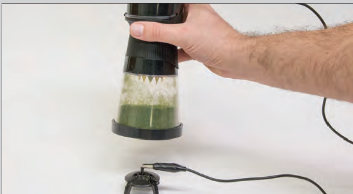
4 Connect alligator clip to anchor. Place anchor near adhesive to activate static application. Turn on Static King and shake in gentle side-to-side motion to apply fibers.
